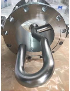
CEPC Collider HOM coupler (1 kW CW) by OTIC and HD
