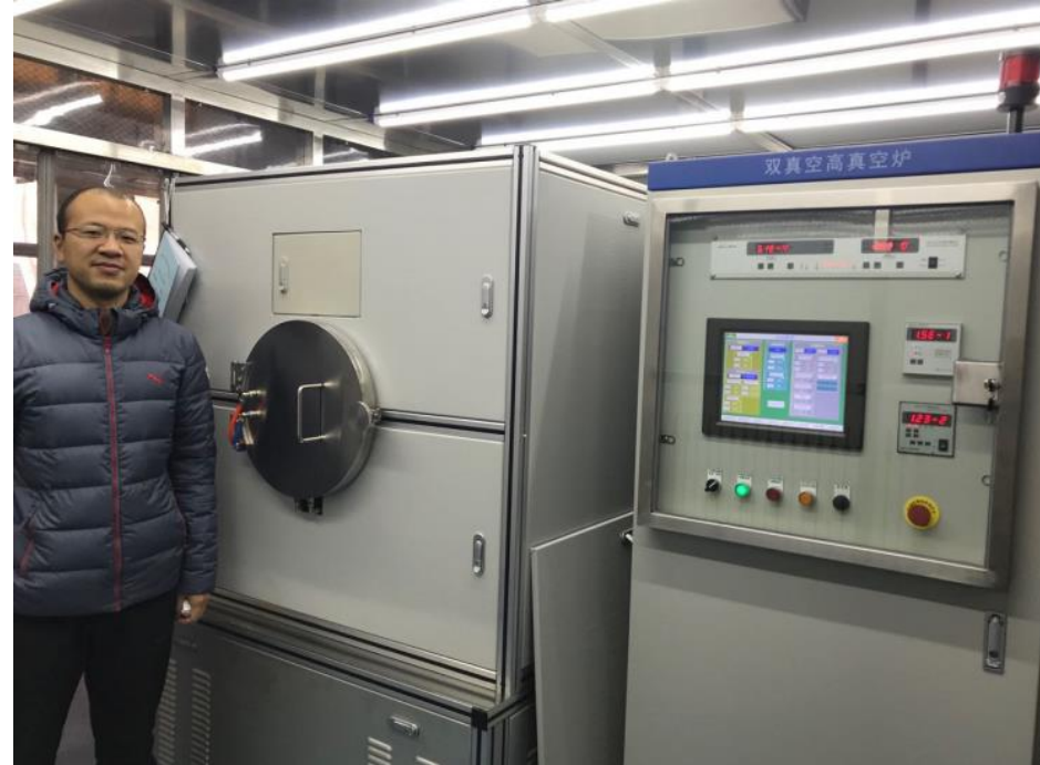
Small furnace for N-doping / N-infusion of 1.3 GHz 1-cavity
