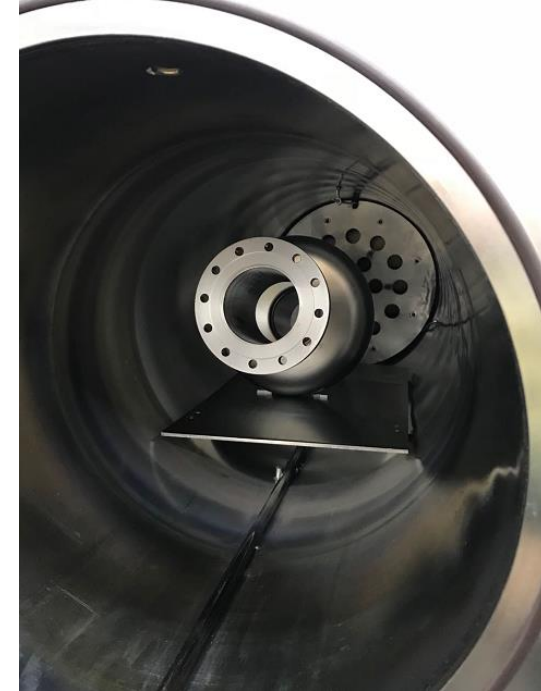
Small furnace for N-doping / N-infusion of 1.3 GHz 1-cavity
