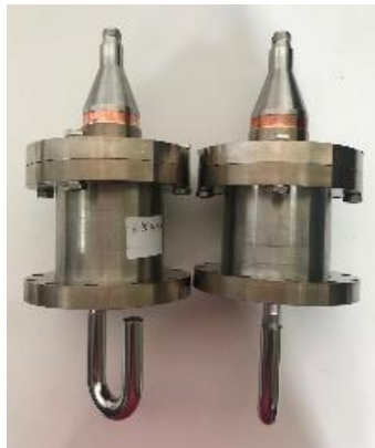
HOM couplers are used for HOM power input and output.
