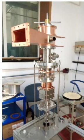
CEPC Booster 1.3 GHz TESLA 9-cell cavity mass production and variable double window coupler by HERT
